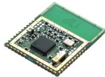
Figure 5 Antenna on same PCB as module (Monopole)
