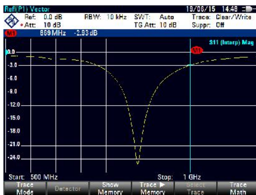
Figure 16 S11 Parameter measurement with VNA
